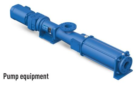
Pumps are used to transport substrate to the equipment and facilities in the biogas plant and away. Biogas plant design allows to access easily to all pumps. Pumps are driven by helical geared motor. Stator has hopper inlet for optimum filling of the pumping chamber, wear-protected, robust universal joint with feeding screw, robust bearing pedestal with close-coupled drive and self-centering of the drive shaft. Pumps have modular design for high flexibility, low life-cycle-costs.
